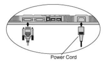
To input the Signal through ADC
